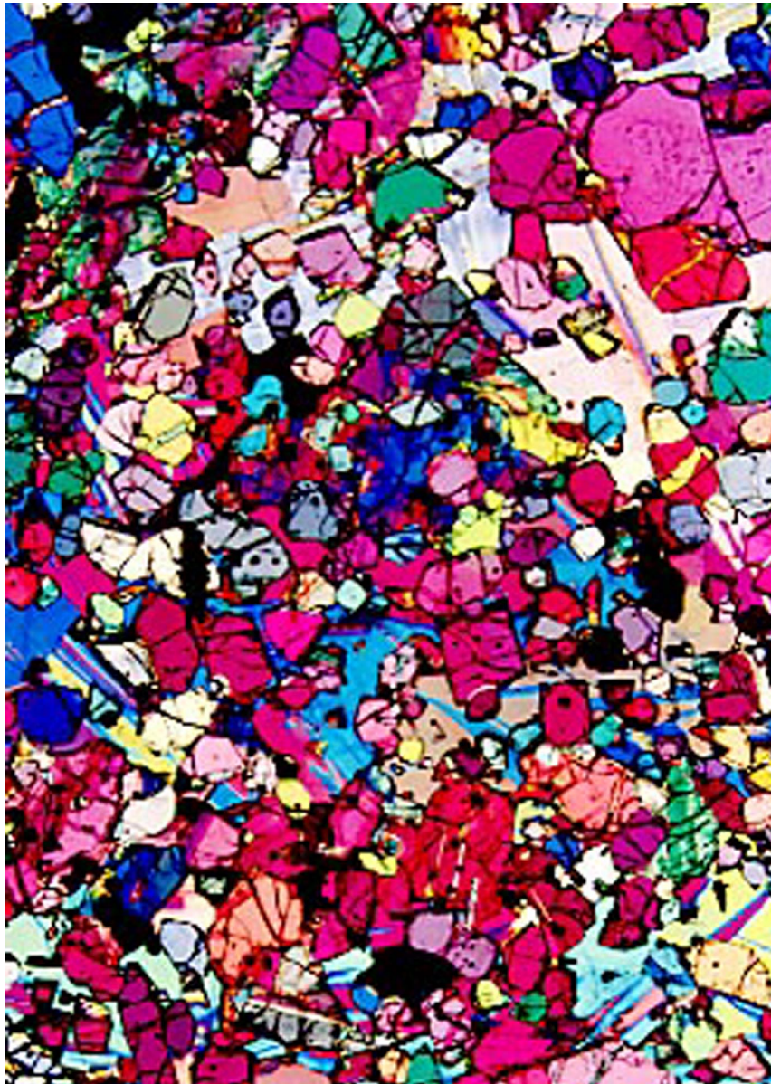
Figure 9. Transmitted polarized light photomicrograph of a lunar basaltic lava sample collected from the Oceanus Procellarum mare region by Apollo 12 astronauts. This sample is 3.15 billion years old and gave the first indications that Granite exists on the moon.
